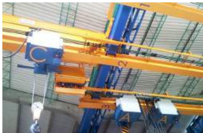
Special design "latching cranes"
