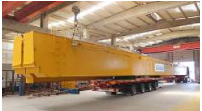
Güralp factory fabricate up to 40 m span of girder
